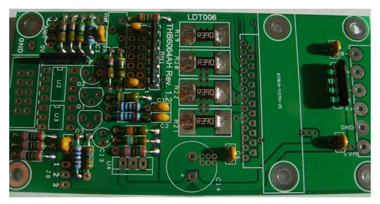
4. Mount the LED's, the longest wire must be in the square hole. Mount the 2 optocouplers also, pay attention for direction, see picture or the silk PDF.
