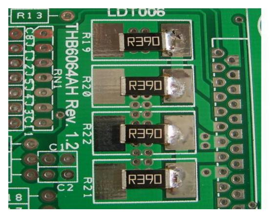
Solder the other sides of the 4 resistors. It should be like the picture below.
