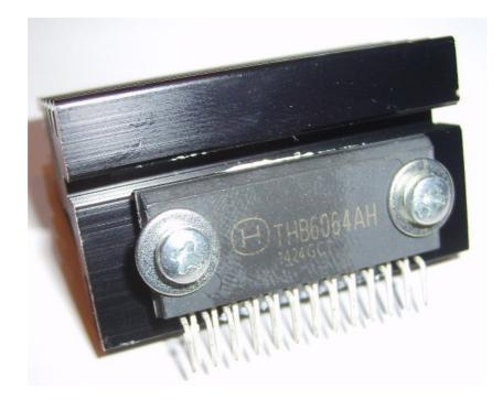
Mount this assembly firmly to the PCB, only solder the pins when everything is aligned properly so that no mechanical stress is introduced.
