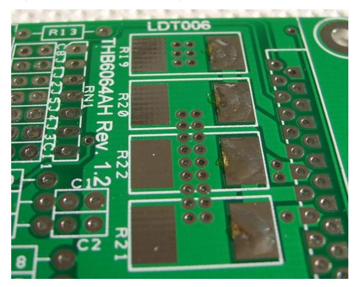
Place the resistor below the solderblob, reheat the solder and shift the resistor so that it is spaced correctly over the 2 pads, result should be like the picture below.
