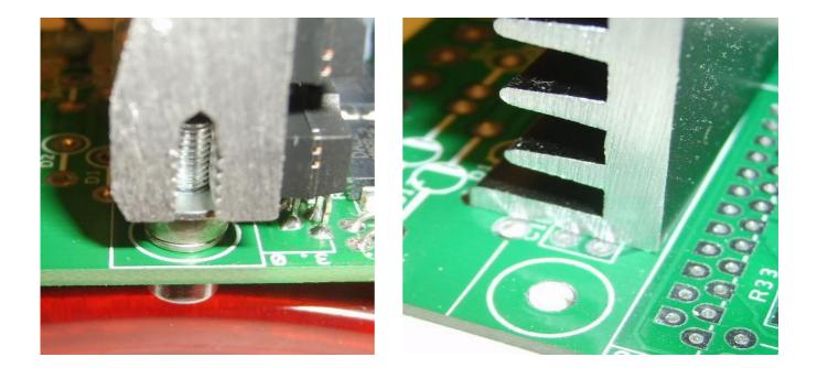
Recently I found a cheap and nice one, the **FISCHER ELEKTRONIK SK 125/50 SA** and the PCB is now adapted for this one.
