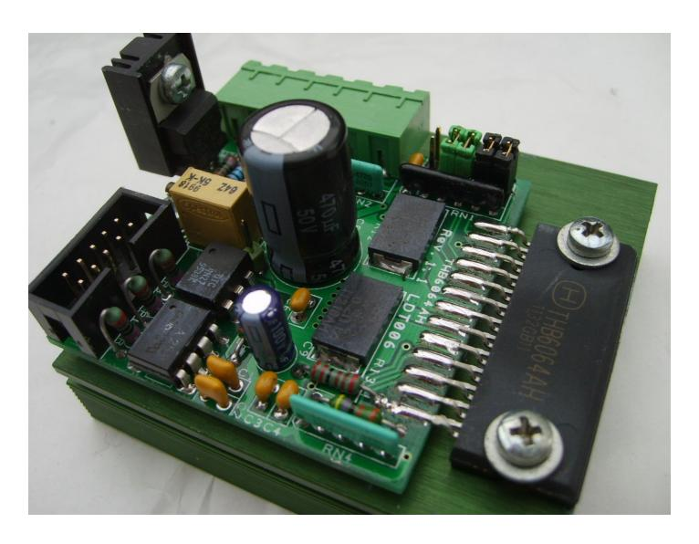
There's enough space between PCB and heatsink if all pins have been cut short, you should be able to slip a PCB (1,6mm thick) everywhere between the 2.
