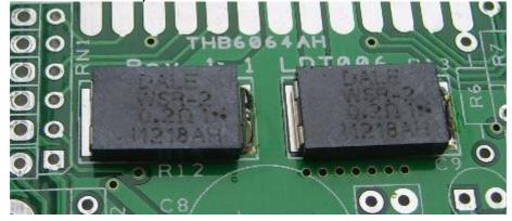
3. Now solder the other side and next install the resistors laying flat, see picture below.
