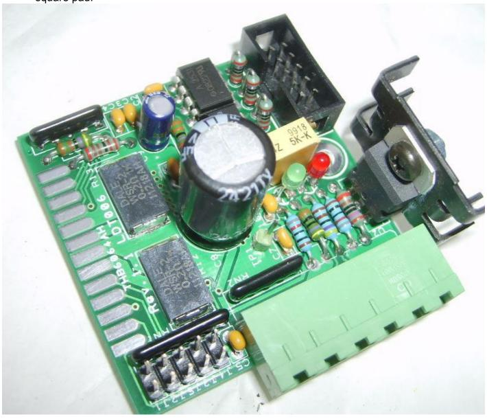
At this point, without the chip installed, do a visual inspection preferably with a magnifying glass. Then apply power, 12-18VDC from a small adapter or a real power supply (40VDC max) but with a 1A fuse in the +VM line. Now the 5V can be checked, the +5v led should be on and the Vref can be measured and adjusted to a low value: 0.4-0.5V. See the connections PDF for the ground testpin and Vref measuring location.
