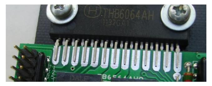
Remove the drive and solder the bottom row of pins.
