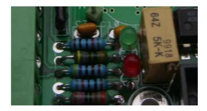
9. There are now 3 components left to install in this sequence: Small electrolytic capacitor, long wire goes in the hole marked with a "+" on the silk or the square pad. Voltage regulator with a small heat-sink, see silk for direction. Big electrolytic capacitor, long wire goes in the hole marked with a "+" on the silk or the square pad.
