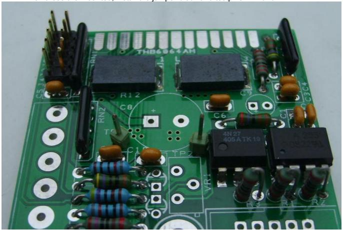
7. Now install the 6 pin motor connector, the flatcable header (see pictures for it's direction) and the 5K trimpot.
