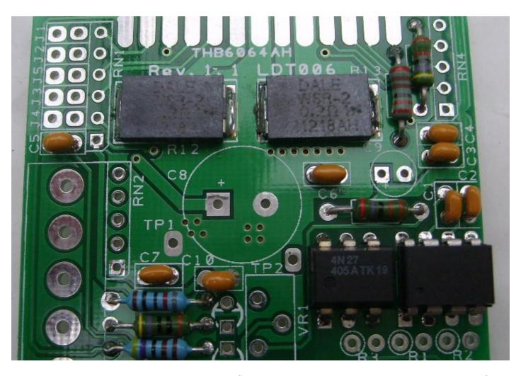
5. Next the resistor arrays, pay attention for pin1, marked with a dot on the array. The pad for pin 1 is the square one.
