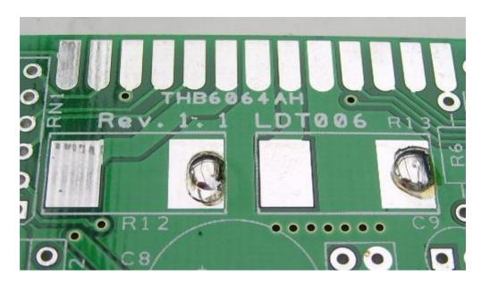
2. Place the resistor to the left of the solderblob, reheat the solder and shift the resistor to the right so that there is some space left to solder the other side.
